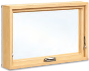
AWNING An awning is hinged to the frame at the top and opens outward. If hinged on the bottom, it’s called a hopper.
